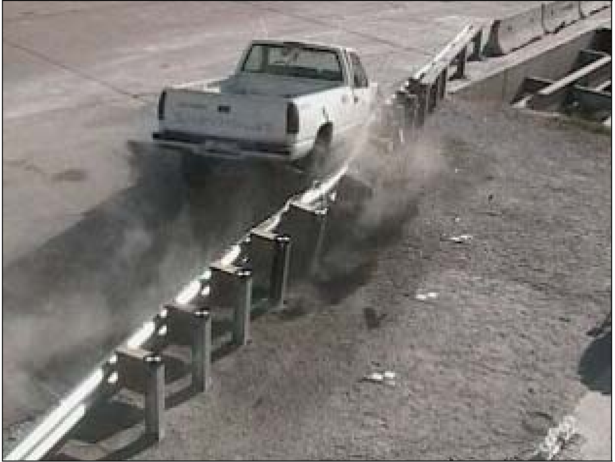
FIGURE 7 Successful Redirection Using the MGS Asymmetrical Transition Element (MWT-5).
