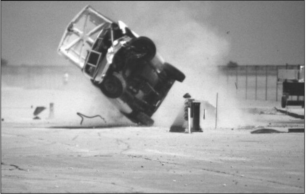
FIGURE 2 Rollover Induced by Transition Element (MWT-2).
