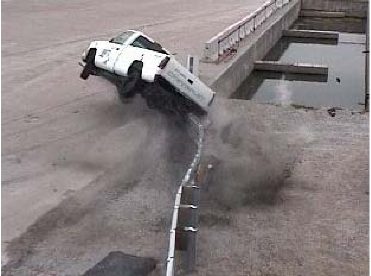
FIGURE 3 Rollover Induced by Increased Stiffness (MWT-3).
