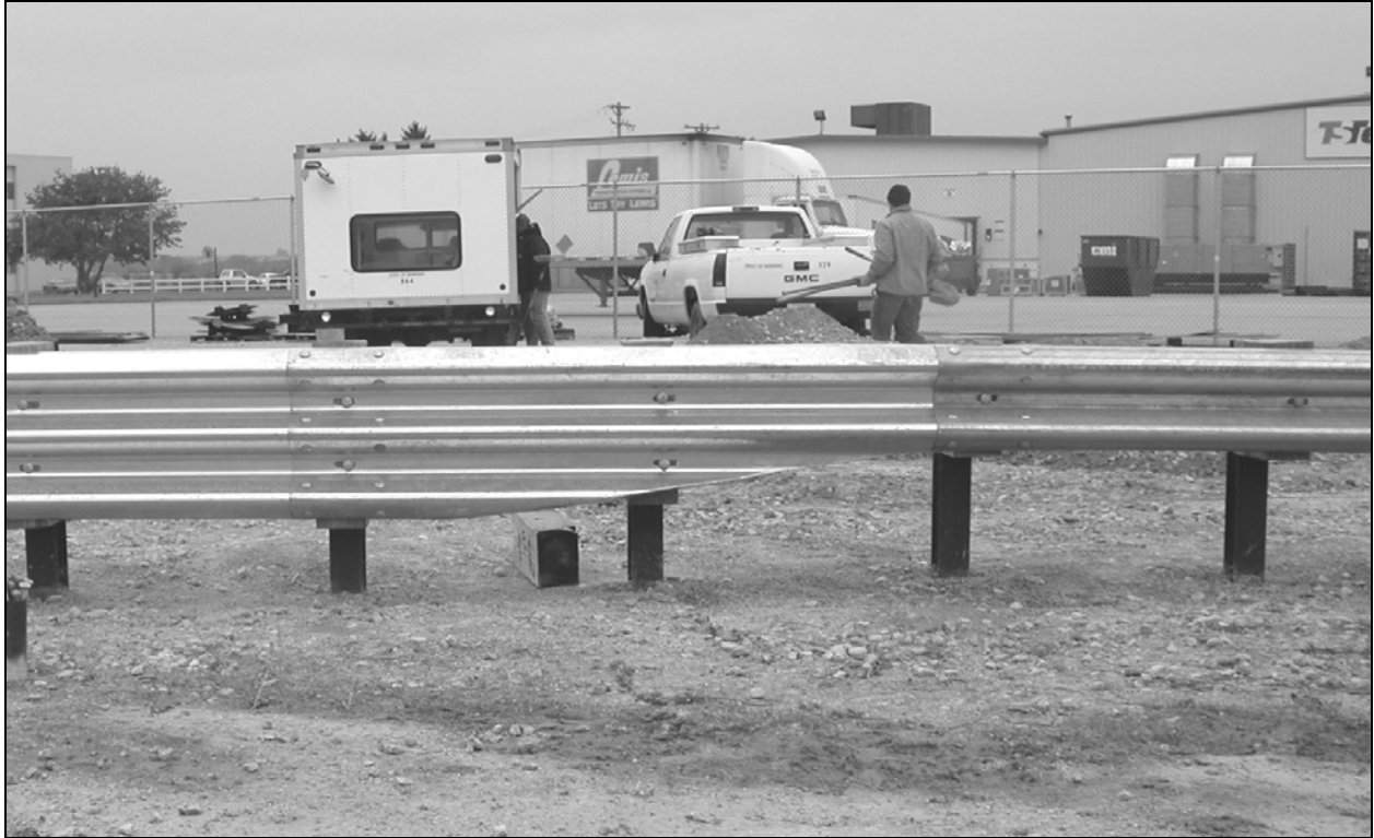
FIGURE 4 Asymmetrical Transition Element Prototype (MWT-4).
