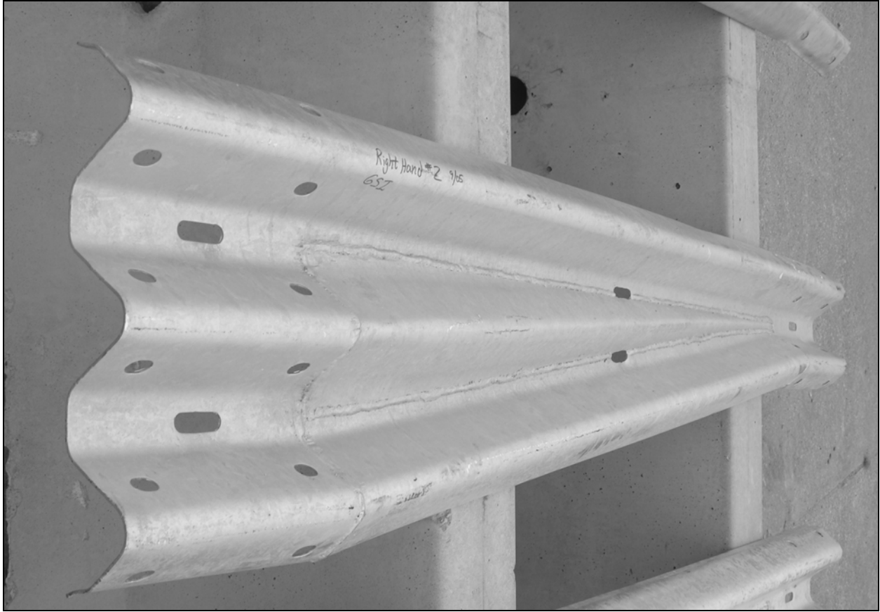
FIGURE 6 MGS Asymmetrical W-Beam to Thrie-Beam Transition Element (MWT-5 & 6).
